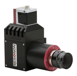
The Pika L is a line-scan hyperspectral camera that covers the visible and near-infrared spectral range (400 – 1000 nm). The Pika L is lightweight and compact, ideal for remote sensing. It can be used with any of Resonon's benchtop, outdoor, and airborne systems, standalone with our software development kit, and integrated into machine vision systems.
