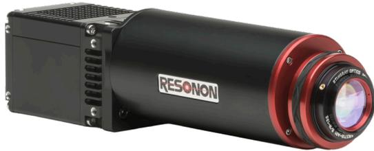
The Pika IR-L is a line-scan hyperspectral camera that covers the near-infrared spectral range (925 – 1700 nm). The Pika IR-L is a high-speed, light-weight infrared imager, ideal for remote sensing applications. It can be used with any of Resonon's benchtop, outdoor, and airborne systems, standalone with our software development kit, and integrated into machine vision systems.
