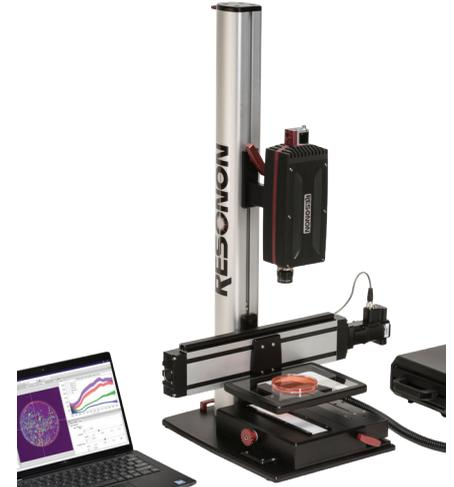
This system allows for illumination from above (Reflectance) or from below (Transmission). A clear sample plate is mounted to the linear stage, which is mounted on the column. The line light is easily transferred between the Reflectance and Transmission configurations.
