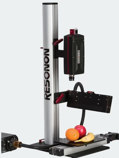
The linear stage holds the sample and translates across the field of view. Used for small samples that are easy to move.
